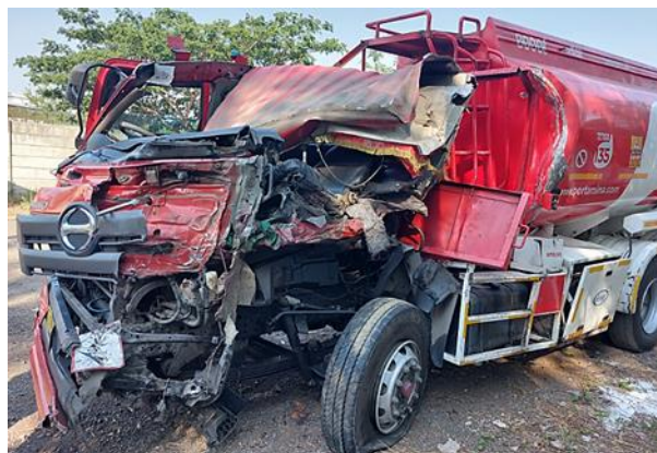
Gambar 6. Tampak samping kiri kabin truk tangki hancur, as roda bergeser ke belakang
