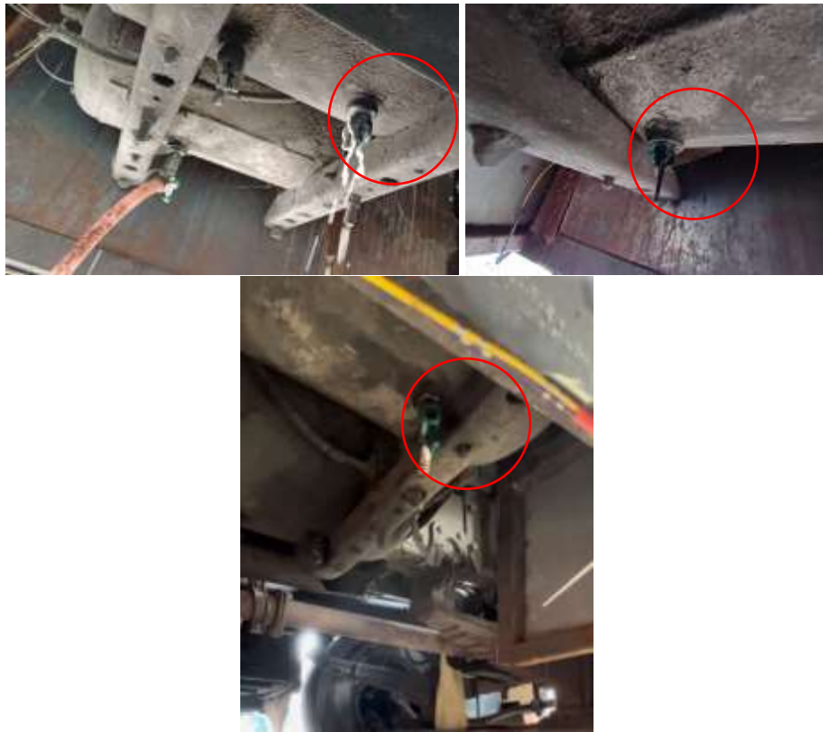
Gambar 13. Kondisi tangki angin ( Reservoir )
