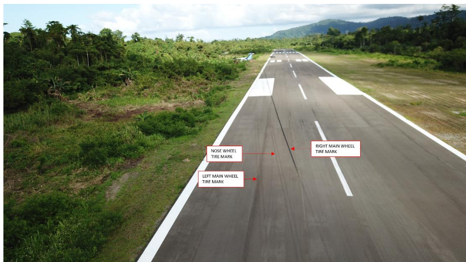
Figure 6: The aircraft tire marks on the runway
